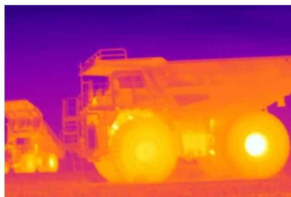
Figure 9. Autonomous thermal inspection of haul trucks in open pit mine [14]
